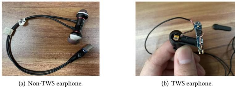
Fig. 21. Non-TWS earphones (a) have visible wires outside. TWS earphones (b) have to rely on manual connections inside the earbud so as to bypass internal circuits.
