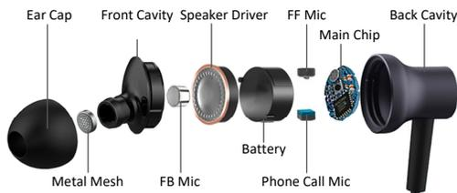
Fig. 19. The structure of an ANC earbud.
